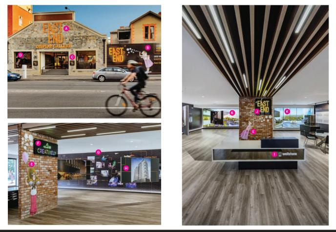
A. Stainless Steel Fabricated Lettering B. Hoarding Signage C. Plaque Signage D. Window Graphics E. Hand Painted Graphics F. Neon Signage G. Wallpaper & Murals H. Hanging Silicone Edged Graphic Fabric Frames I. Acrylic Lettering J. Acrylic Lightbox K. Silicone Edged Graphic Fabric Frame Lightbox
